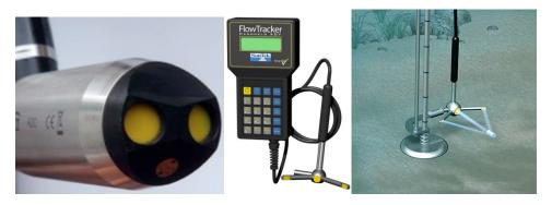
The FlowTracker is based off of Sontek's ADV design with a side looking sensor. It measures a very small space of water four inches away from the center transducer. This offset requires the use of an offset bracket on the wading rod to try to get the sampling volume closer to the position of the rod in the measured vertical. The FlowTracker is kept perpendicular with the tagline and the device measures any angles and corrects for them automatically in the software.
